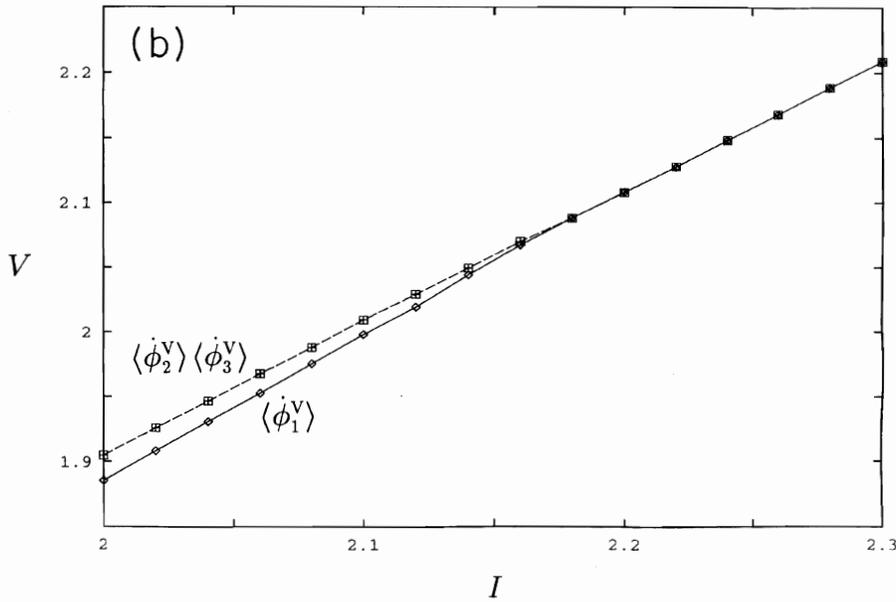
FIG. 11. (a) A row of junctions. The critical current of each junction is indicated (high disorder). (b) The corresponding  $I$ - $V$  curves, showing a transition to a desynchronized state. The junction resistances are all equal to unity. After the transition, two of the vertical junctions continue to be frequency locked in this example. Note that for lower levels of disorder no fork in the  $I$ - $V$  curve would exist.
