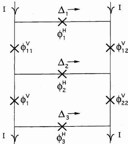
FIG. 8. The double plaquette. The vertical junctions in the first row are denoted by  $\phi_{11}^V$  and  $\phi_{12}^V$ , and those in the second by  $\phi_{21}^V$  and  $\phi_{22}^V$ . The horizontal junctions are  $\phi_1^H$ ,  $\phi_2^H$ , and  $\phi_3^H$ .  $\Delta_1$ ,  $\Delta_2$ , and  $\Delta_3$  represent the induced currents shunted across the horizontal junctions.
