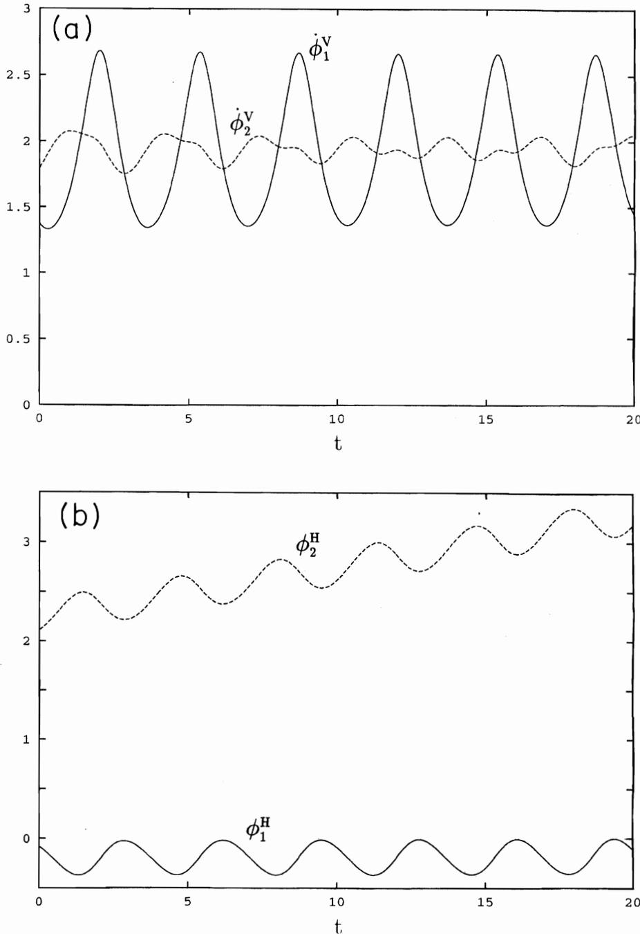
FIG. 5. Desynchronized state of the plaquette:  $I_{c_1}^V = 1.0$ ,  $I_{c_2}^V = 0.4$ ,  $I_{c_1}^H = 0.3$ ,  $I_{c_2}^H = 0.01$ ,  $I = 2.0$ , and all resistances equal to unity. (a) The voltage oscillations of the vertical junctions  $\dot{\phi}_1^V(t)$  and  $\dot{\phi}_2^V(t)$  are unlocked. (b) The horizontal phase  $\phi_2^H(t)$  displays linear growth on average.
