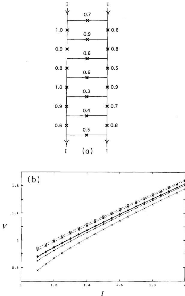
FIG. 13. (a) A  $6 \times 2$  array. The critical current of each junction is indicated (moderate disorder). (b)  $I$ - $V$  curves, demonstrating that the vertical junctions in the six rows have different oscillation frequencies (two of these frequencies are close in value and difficult to distinguish in the plot). Within each row, the vertical junctions are frequency locked. Intra-row locking would be destroyed at higher levels of disorder (not shown).
