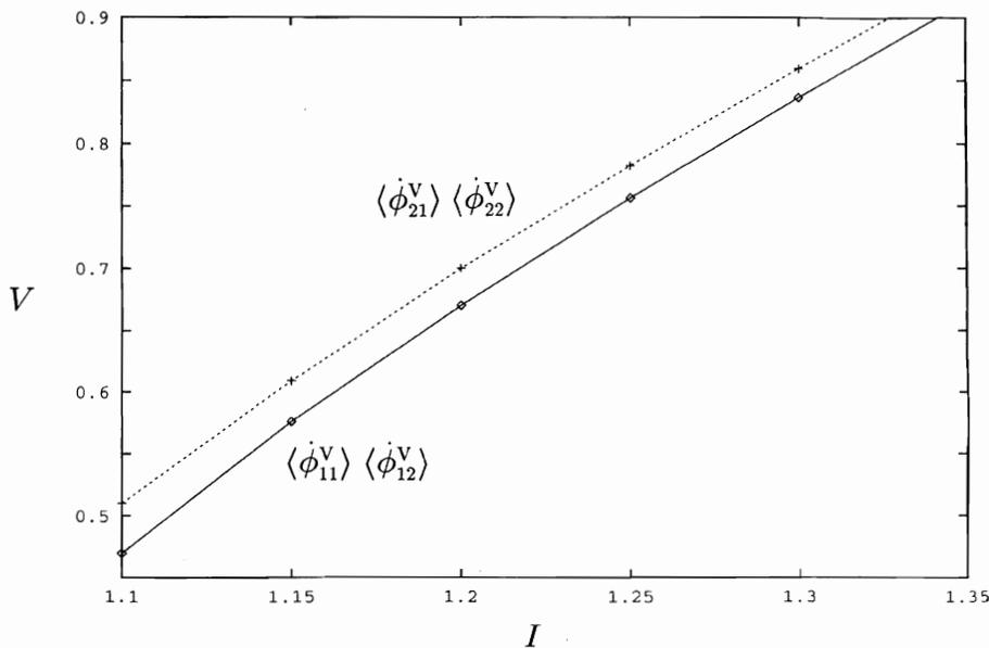
FIG. 12.  $I$ - $V$  curves for the double plaquette with weak disorder ( $I_{c_{11}}^V = 1.00$ ,  $I_{c_{12}}^V = 0.99$ ,  $I_{c_{21}}^V = 0.98$ ,  $I_{c_{22}}^V = 0.97$ ,  $I_{c_1}^H = 0.99$ ,  $I_{c_2}^H = 0.97$ ,  $I_{c_3}^H = 0.98$ ). The vertical junctions in the same row are frequency locked, but the characteristic frequency of each row is different.
