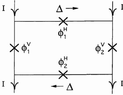
FIG. 3. The plaquette. The phase differences across the vertical and horizontal junctions are denoted by  $\phi_1^V$ ,  $\phi_2^V$  and  $\phi_1^H$ ,  $\phi_2^H$ , respectively. Current  $I$  is imposed at the top and removed at the bottom;  $\Delta$  is the induced current shunted across the horizontal junctions.
