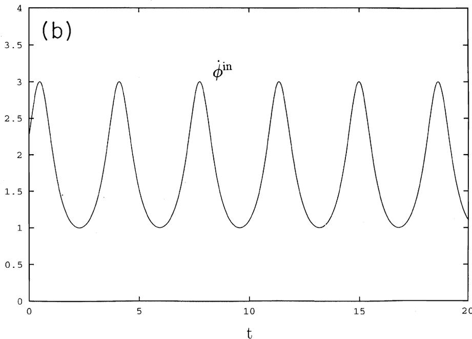
FIG. 2. In-phase state of identical-junction array. (a) shows the direction of current flow, with all horizontal junctions inactive and all vertical junctions having the same functional waveform  $\phi^{in}(t)$ ; (b) representative time series for  $\phi^{in}(t)$ .
