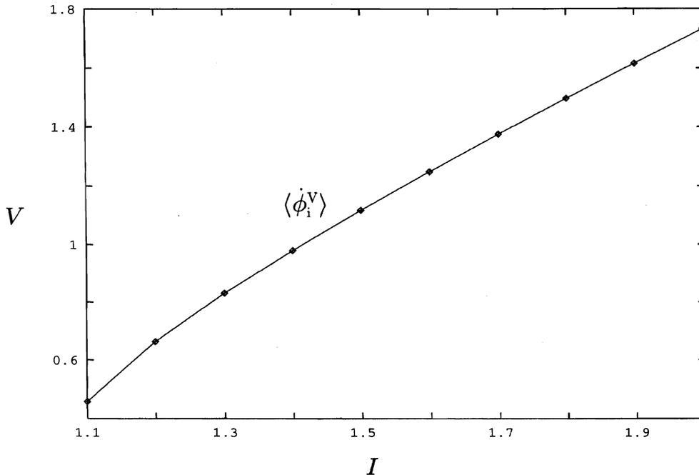
FIG. 9.  $I$ - $V$  characteristic of an  $N \times M$ , identical-junction array in the in-phase state. The time-averaged voltage of the individual junctions  $\{\langle \dot{\phi}_i^V \rangle\}$  is shown. In this state all vertical junctions  $\phi_{ij}^V$  display the same  $I$ - $V$  behavior; the horizontal junctions  $\phi_{ij}^H$  are inactive. For different initial conditions (leading to states related to, but distinct from, the in-phase state), the same  $I$ - $V$  behavior results.
