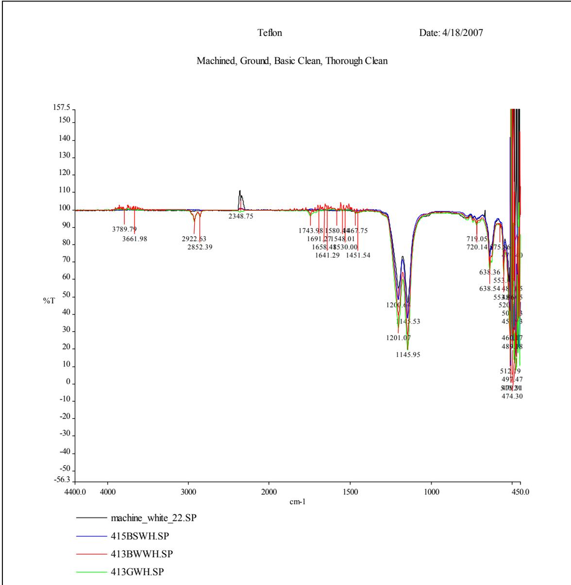
Figure R3. Elimination of CO<sub>2</sub> from FTIR spectra for PTFE
