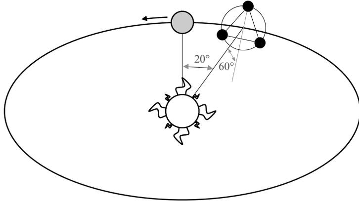
**Figure 1.1:** Each of the three spacecraft that comprise LISA independently orbit the sun. The orbits are such that the spacecraft form a stable equilateral triangle with sides of  $5 \times 10^6$  km. The plane of this triangle is always inclined  $60^\circ$  away from the sun-earth orbital plane, and it trails about  $20^\circ$  behind the orbit of the earth.
