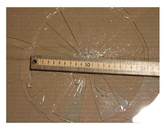
Above and Below: an example of measuring the radius of shattering. Note that the breakage is not completely circular. The two radii measured will be averaged together for an estimated radius of shattering of this particular break.
