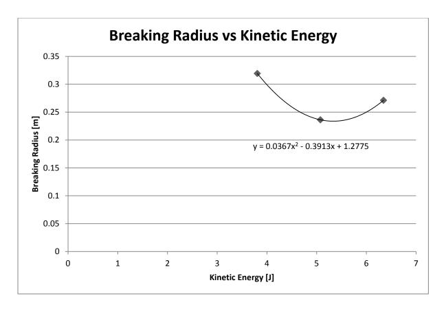
When compared to the kinetic energy of the ball, we see that while it is possible that there exists a quadratic relationship between the energy of the falling object and the radius of the radial shattering, it is not the one that was expected. Admittedly, assuming a quadratic relationship from three data points is not necessarily sound, and this experiment should be expanded in order to better understand the behavior.
