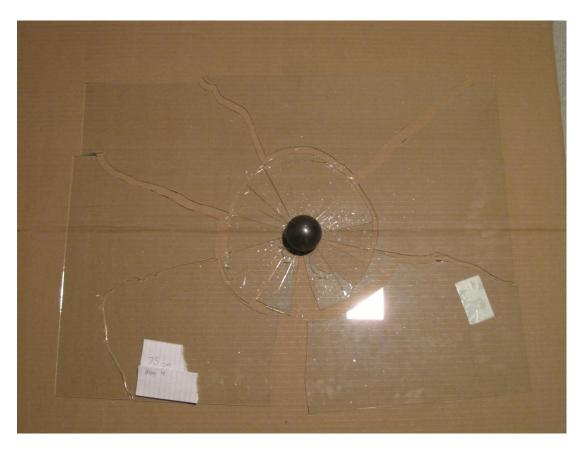
Example of a breakage from 75 [cm]. Note the breakage pattern, with an interior area of radial shattering and an exterior area of less well defined breakage.
