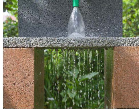
Figure 5: A demonstration of pervious pavement. Source: Wikipedia user JJ Harrison
