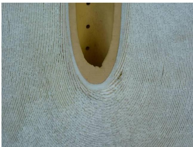
Microfiltration tube cutaway.
