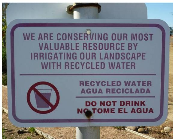
Required signage to mark non-potable reuse
