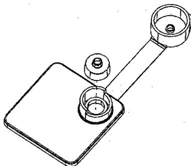
Figure 3: Lens case assembly
