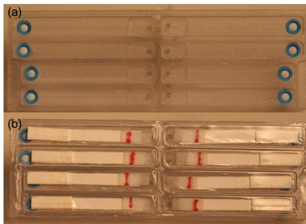
Figure 16: Lateral flow strip chamber testbed. (a) Empty lateral flow strip chambers, showing embedded hydrophobic barriers (blue). (b) Lateral flow strip chambers with lateral flow strips sealed by polycarbonate film. The red line on the conjugate pads is the lateral flow conjugate that has been dispensed and dried onto the conjugate pad.
