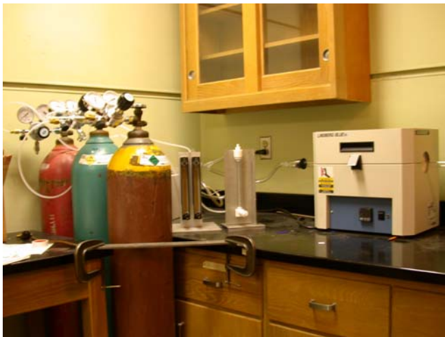
Figure 1. Our growth apparatus. From left to right: hydrogen, methane and argon bottles, Gilmont flowmeters for argon, methane and hydrogen, Lindberg Blue tube furnace.
