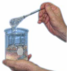
Clearco 100,000cSt is a High Viscosity Silicone that has a viscosity similar to molasses
