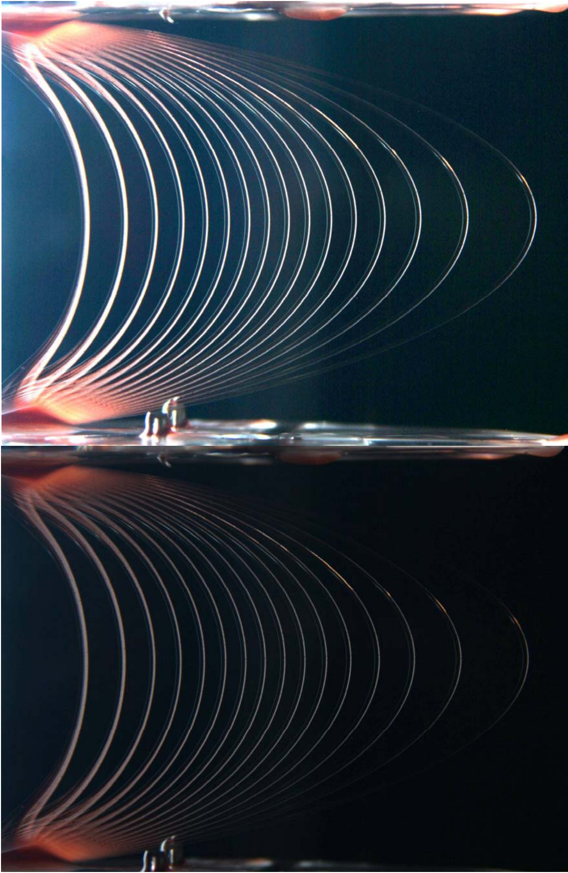
Figure 4.11: A typical falling filament before and after Photoshop enhancement. The strobe speed is 0.7 seconds. A high resolution version of the enhanced picture is available on the CD.
