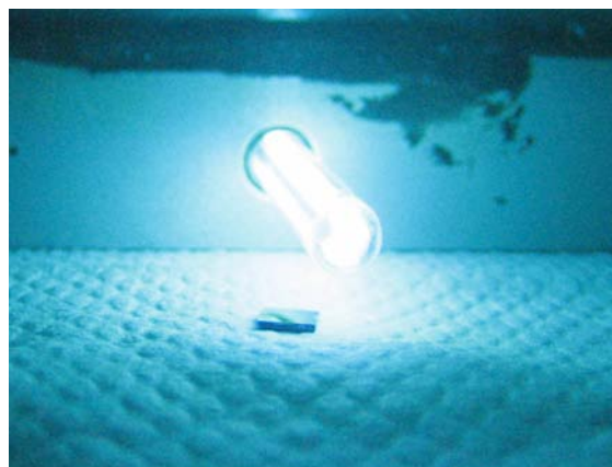
Figure 4.1: An image of a small UV-Penlamp taken while it is on. Obviously the wavelengths that generate the ozone are not visible, but the emitted spectrum extends into the violets. These lamps should never be viewed with the naked eye.
