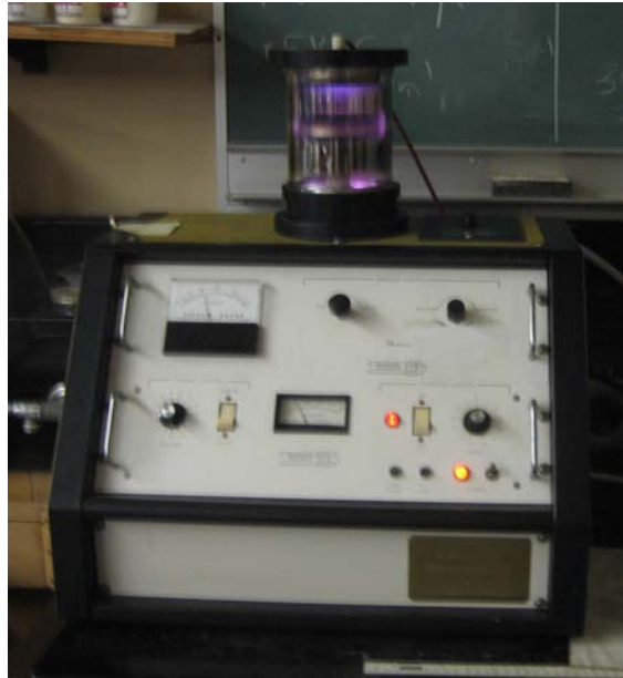
Figure 4.3: The Hummer II DC Plasma Etcher that we used. The purple color of the plasma in the chamber at the top of the machine is characteristic of Argon.
