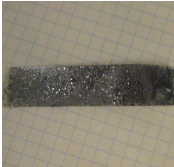
(b) A piece of standard scotch tape that has been almost completely covered by flakes of graphite after repeated folding.
