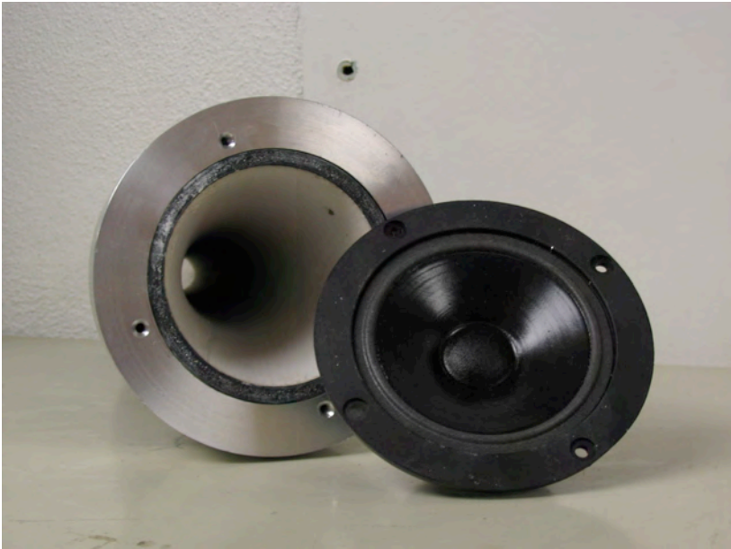
Figure 3.3: Exponential Horn with Speaker Mount and Speaker
