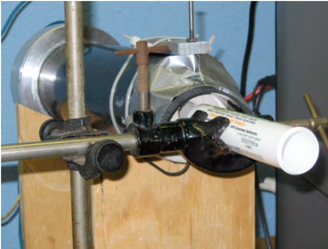
Figure 3.9: Measurement of Pipe Free-field Impedance Spectrum
