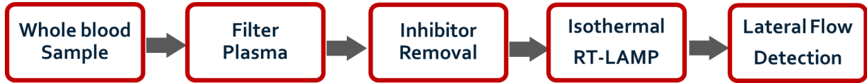
Figure 38. DENV Full Process Execution. Starts with whole blood sample preparation followed by filter plasma via plasma separation device then RT-LAMP isothermal amplification and lateral flow detection.
