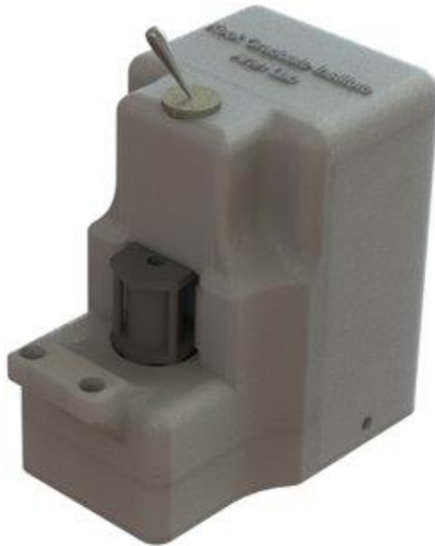
Figure 2.1: The single pump microfluidic blood handling system is a 3D printed device that features a single pump head.
