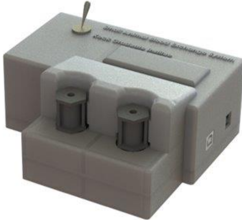
Figure 2.2: The dual pump microfluidic blood handling system is a 3D printed device that features 2 independent pump heads.
