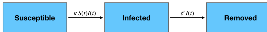
Figure A1: Visualization of the SIR model described by (A.2). Parameter \kappa is the rate of infectivity and \ell is the rate of removal.
