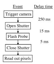
FIG. 1. A flowchart of the timing associated with taking a single image used for absorption imaging. The full exposure time of the camera is 700 ms, but a mechanical shutter mounted on the front of the camera is closed during the vast majority of this time, over which essentially no noise from dark current accumulates.
