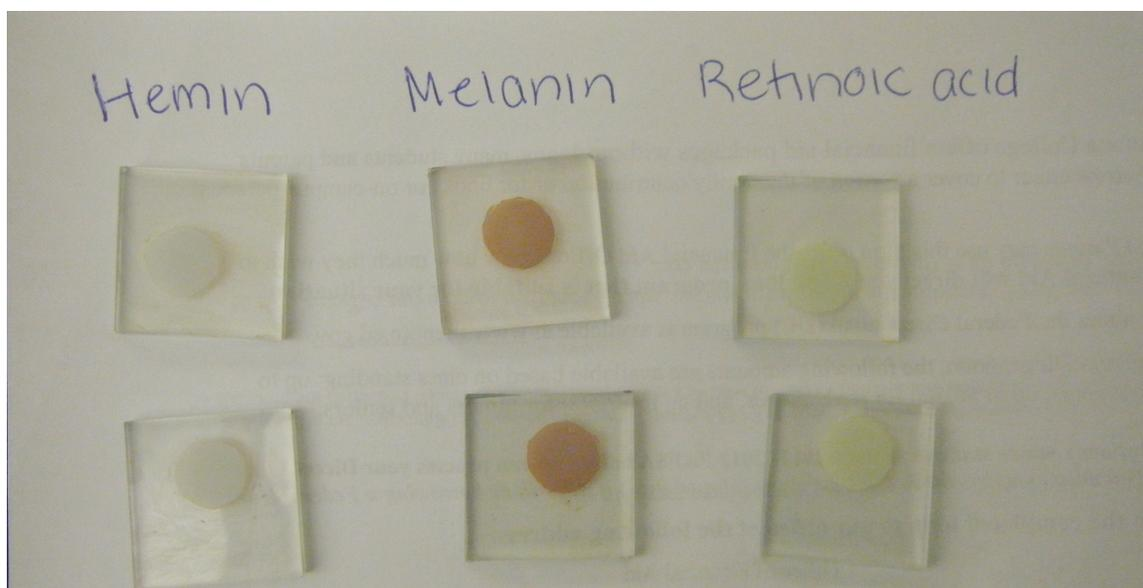
**Figure 9.** Slides with  $\text{TiO}_2$  after immersion in solutions of hemin, melanin, or retinoic acid for two days. Slides were removed from dye and rinsed with water followed by rinsing with ethanol and drying with compressed air.
