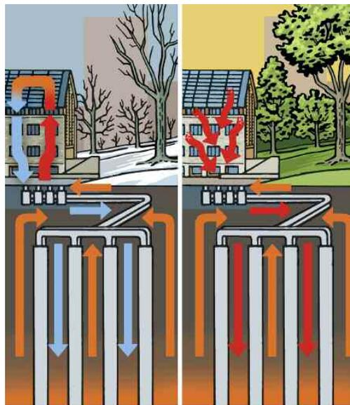
Figure 5. Diagram of Kroon Hall's open loop wells in winter (left) and summer (right), Illustration by Gregory Nemeec.
