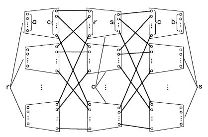
Fig. 1. The interconnection of subnetworks in three stages to form a network. The thick lines joining subnetworks represent identifications of inputs and outputs to form links, not edges.
