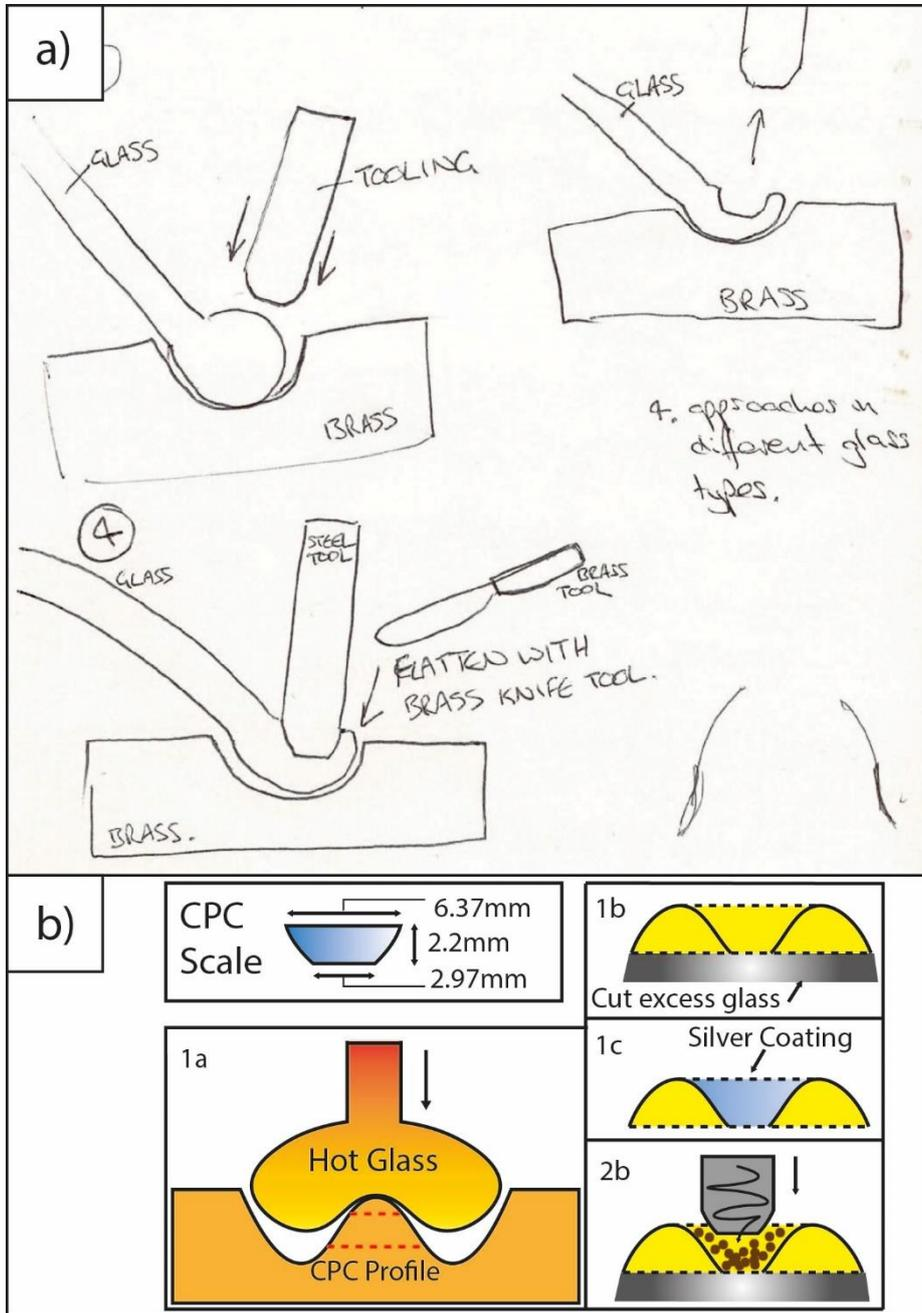
Fig. 2 a) Sketch with notations for an improvised lampworking technique. b) Scientific visualisation of cross-sectional flow diagram outlining developed glass process (caption would be used to explain steps in scientific paper)
