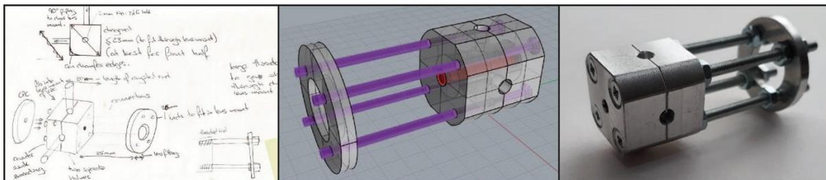
*Fig. 4 Laser chamber design developed through collaboration with physics academics and technicians: sketch, CAD & machined parts*
