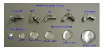
FIG. 8. (Color online) The photo shows many of the link designs that were fabricated and tested. Each design was created from a single piece of acrylic.
