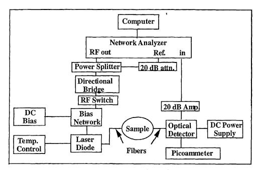
Figure 1. Schematic of the frequency-domain photon migration instument.
