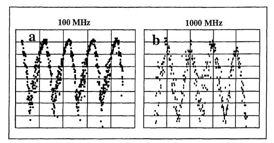
Figure 2. Source modulation at a dc bias of 254 mA and a) 100 MHz and b) 1000 MHz. The vertical scates in a) and b) are 100 and 50 mV/div. respectively. The corresponding horizontal scales are 10 and 1 ns/div. respectively.
