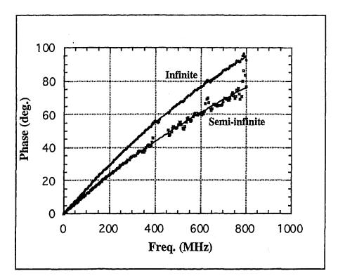
Figure 3. Phase vs. frequency response for 2% Intralipid and 1  $\mu$ g/ml NiSPC tissue-simulating solutions of two geometries. In both cases, the effective source-detector separation was 7.0 mm. The curves represent best fits to the data.
