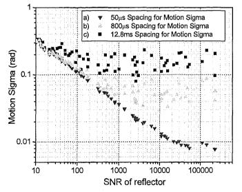
Figure 6 - System phase noise as a function of OCT signal for a) 50µs, b) 800µs and c) 12.8ms
