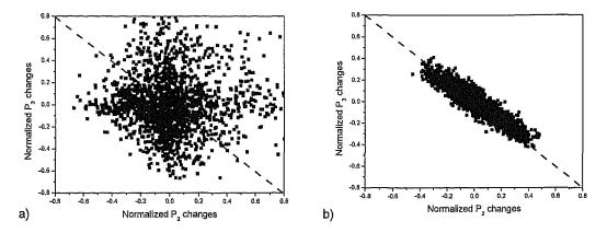
Figure 4 – Correlation plots of normalized changes in power spectrum components for cases with motion sigma of 0.22 radians: a) phase accuracy limited measurements at 50µs and b) system motion noise limited for 2ms Dashed line corresponds to expected form for negative correlation.
