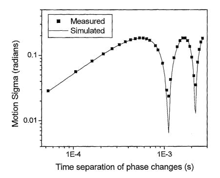
Figure 8 – Phase noise measured from 910Hz Piezo oscillated sample mirror. Simulated motion sigma for 910Hz sinusoidal oscillation of amplitude 0.13 radians overlaid over data.
