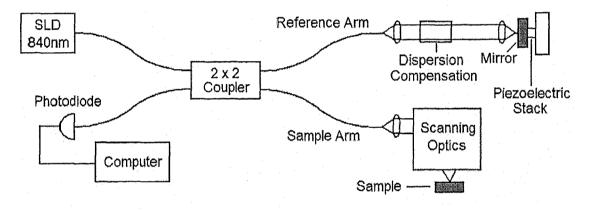
Figure 1 - Schematic of en face phase sensitive OCT system
