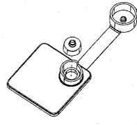
Figure 3: Lens case assembly
