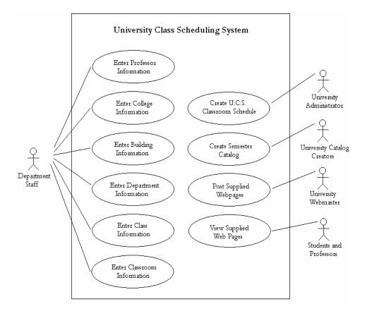
Fig. 1 Use Case Diagram of the UCS
