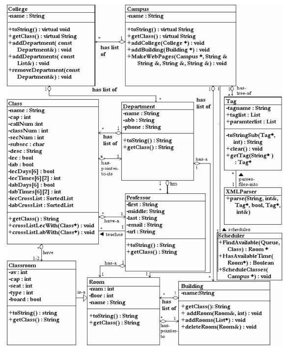
Fig. 6 The Class Diagram of the UCS
