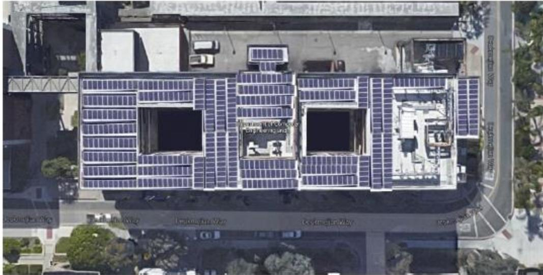
FIGURE 27: Proposed PV system on the roof of the ECS building.
