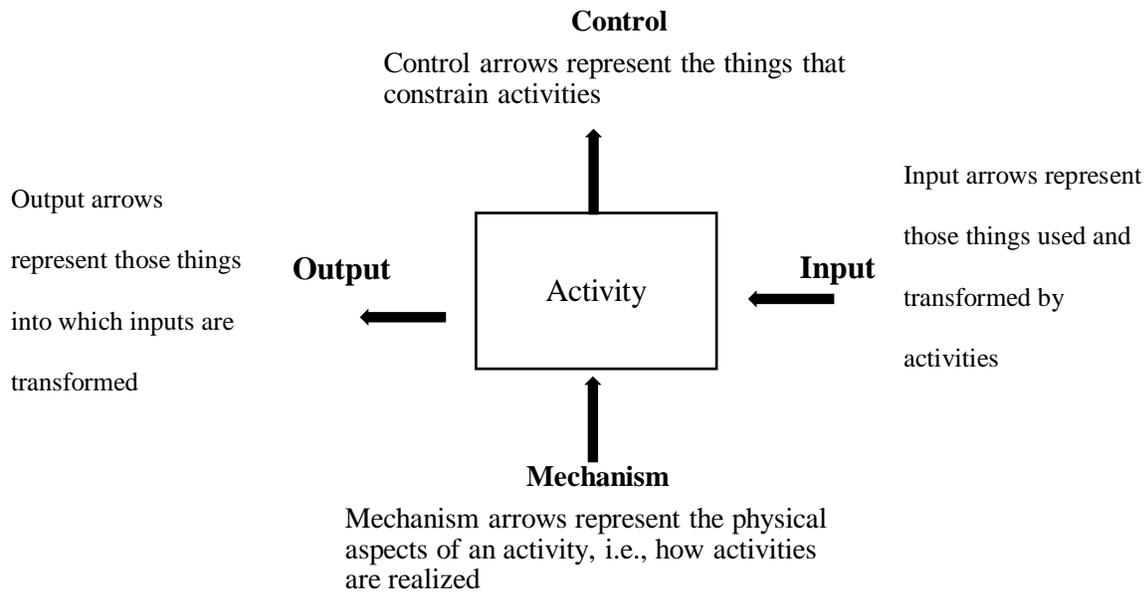
*Figure 1.* The basic concepts of the IDEF0 method.
