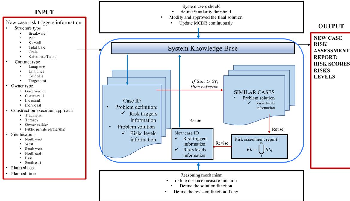
Figure 3. The proposed RLPF process
