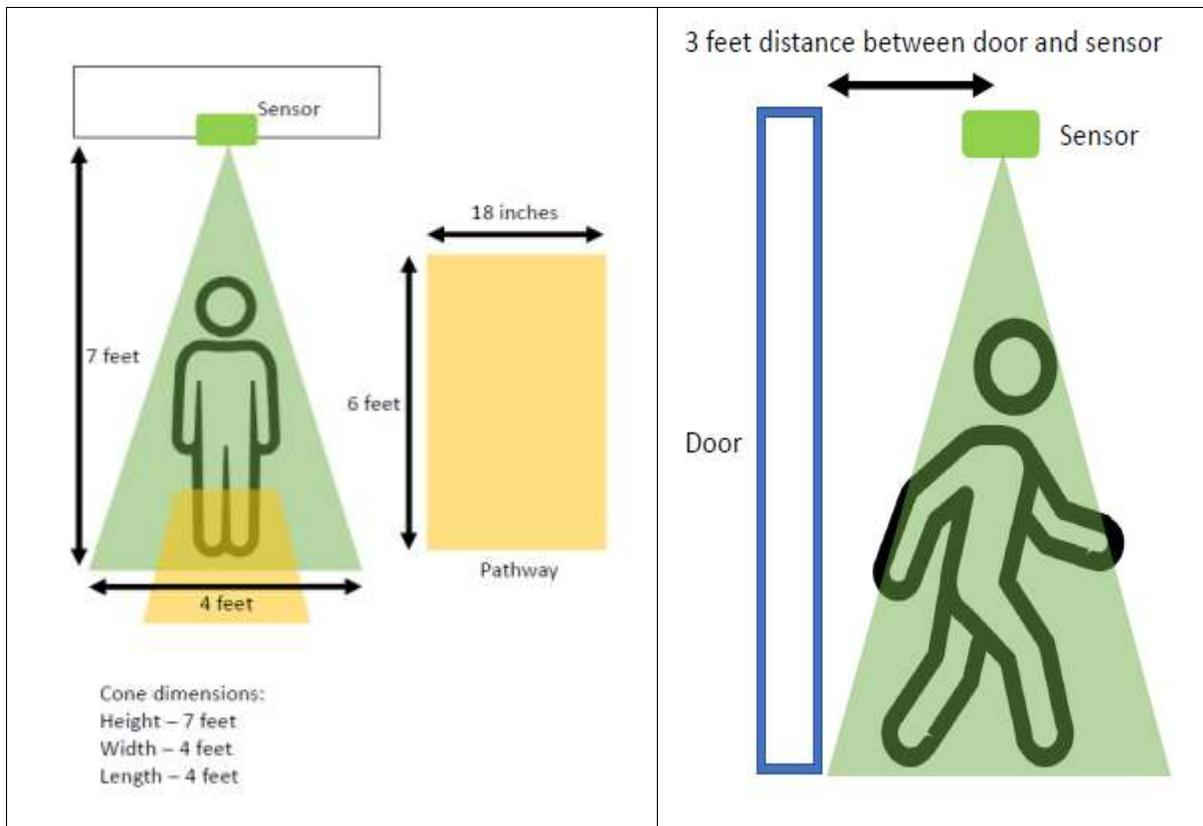
**FIGURE 21: SENSOR PLACEMENT**
