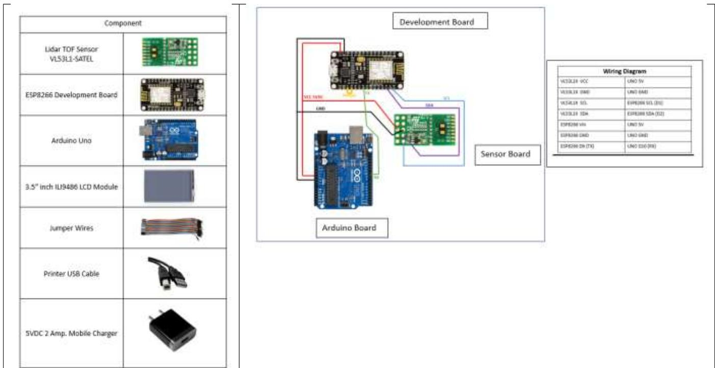
FIGURE 19: SENSOR COMPONENTS AND THE BUILD
