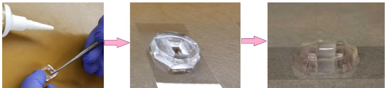
Figure 3.7. To set up the PDMS mold for an experiment, we first attached the PDMS mold to a glass coverslip using a silicon glue. Next, we used small cut coverslips to separate the compartments from each other. We then added the collagen mixture to the middle compartment and let it form in the incubator.
