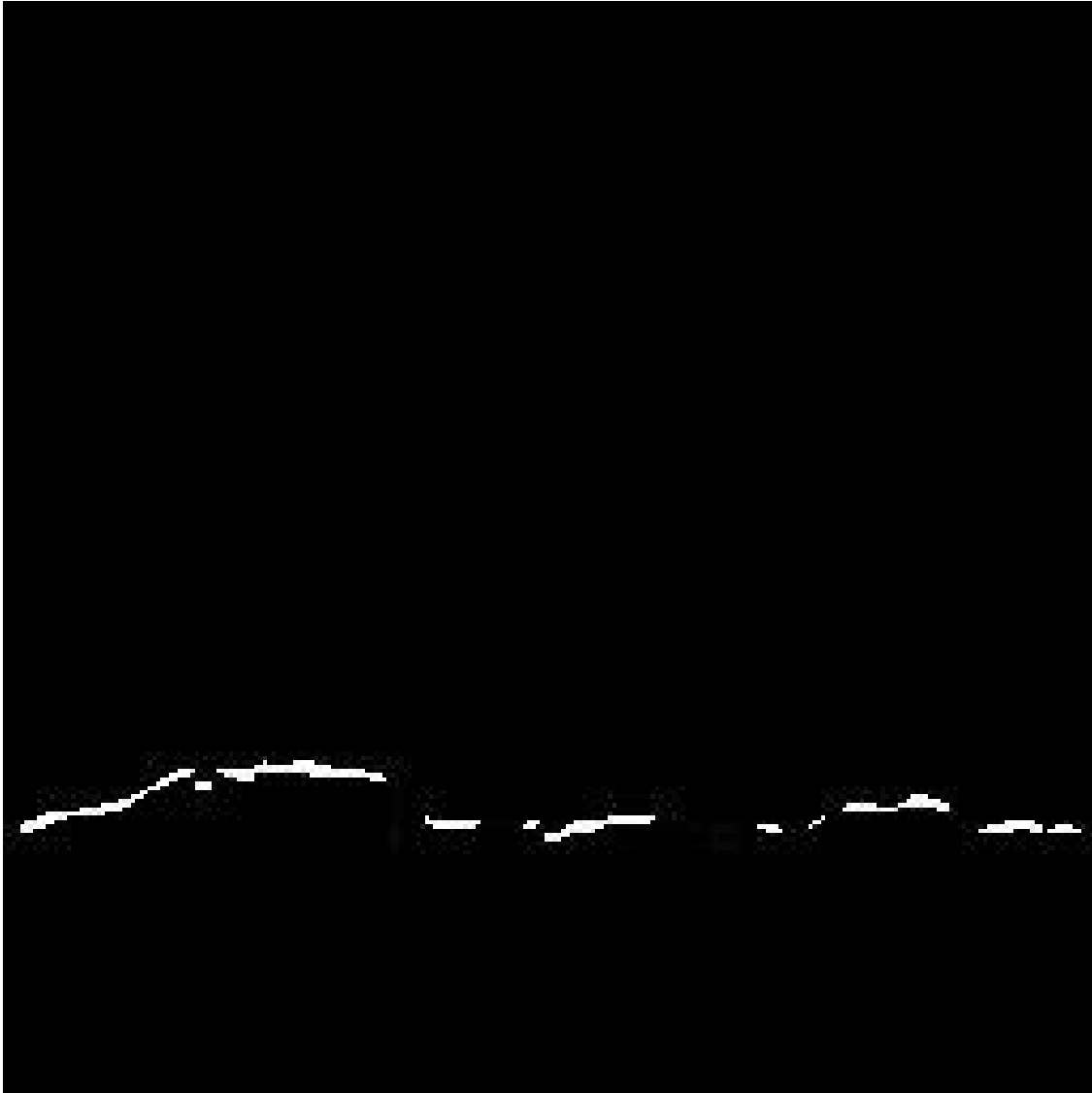
Figure 7.15: Image of Upper Portion of Edge Map for Pavement Crack
