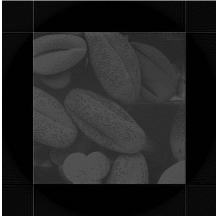
Figure 8.64: Reconstructed Image Using Filtered Back Projection and the Shepp-Logan Filter
