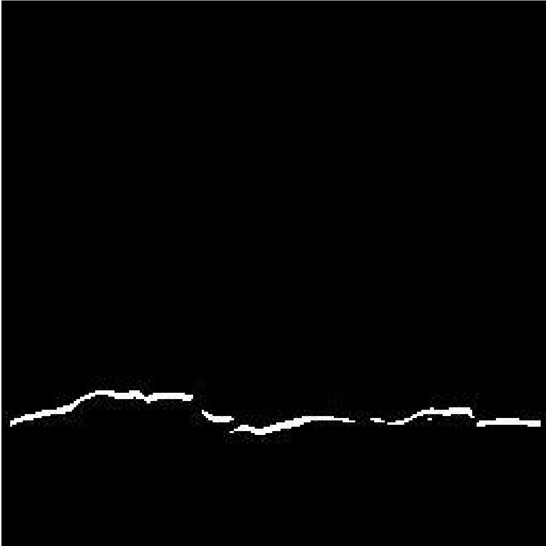
Figure 7.16: Image of Lower Portion of Edge Map for Bridge Deck Crack
