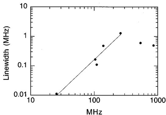
FIG. 1. GAWBS linewidth (FWHM, full width half-maximum) as a function of spectral position. The line is a single exponential fit of slope 2.06 to the first 5 data points. The lowest frequency point at  $\sim 22$  MHz was taken from a sample displaying the narrowest observed signal.
