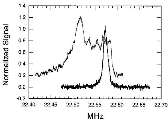
FIG. 2. GAWBS signals from two samples from the same spool of Corning "Flexcore 1060." The narrow resonance has a FWHM of 11 kHz.
