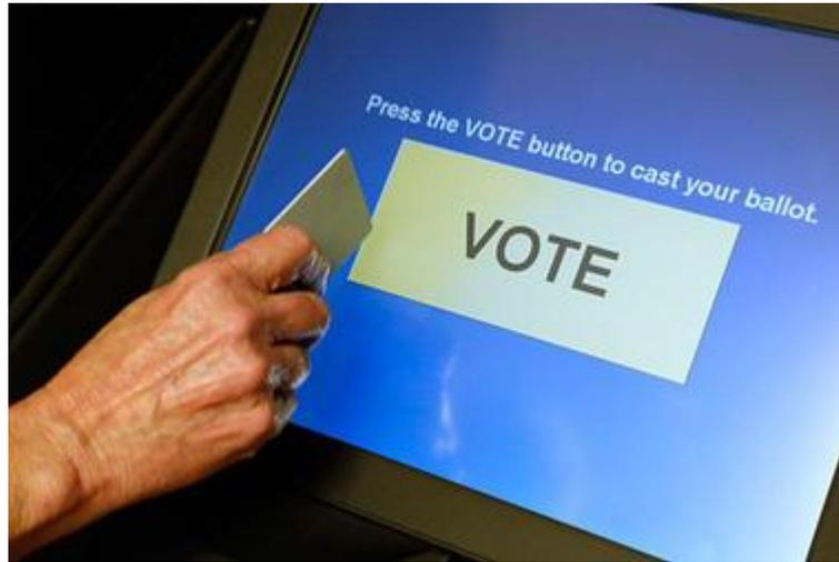
FIGURE 2 THIS IS AN EXAMPLE OF A NEWER DRE MACHINE. THE INTERFACE IS NOW GRAPHIC AND IS TOUCHSCREEN.<sup>31</sup>
