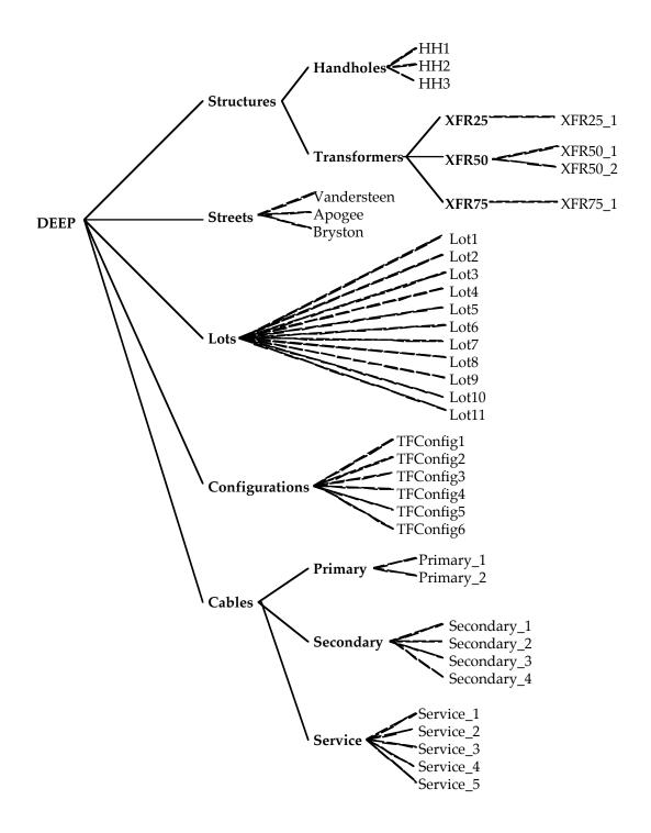
**Figure 3.** The inheritance lattice (or object tree) in the DEEP KBES (Dym, Summers et al., 1995).
