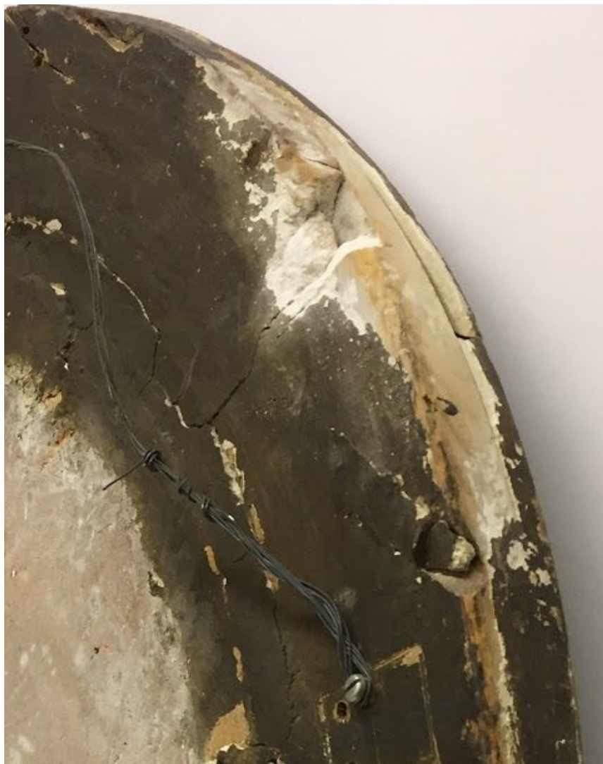
Figure 5: Calligraphic Roundel, Large section of plaster loss in the frame, Reverse. Source: Josephine Ren.
