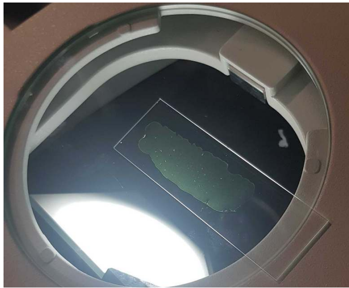
Figure 7. Illumination of glass slide from below
