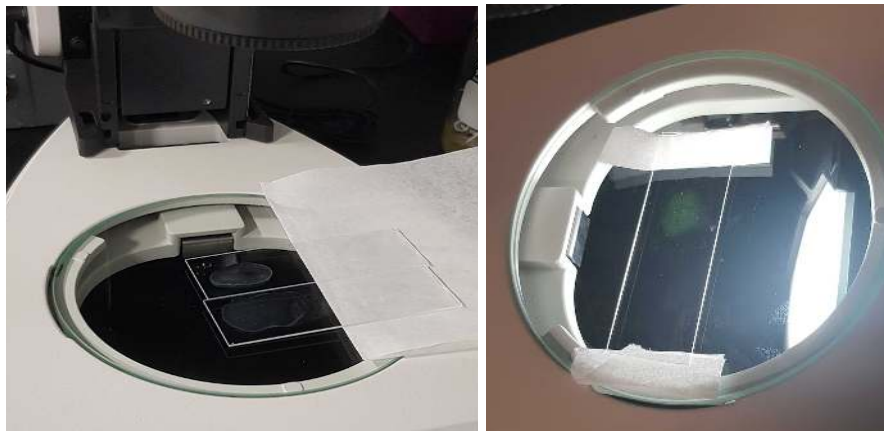
Figure 6. Glass slides on microscope: either half (left picture) or partially (right picture) on kimwipe
