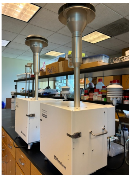
Figure S 3. MesaLabs PQ200 Ambient Air Particulate Sampler side exterior
