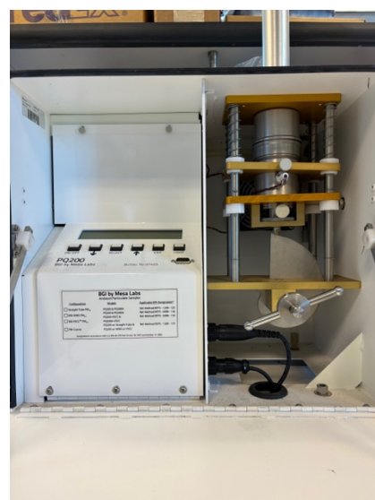
Figure S 2. MesaLabs PQ200 Ambient Air Particulate Sampler interior
