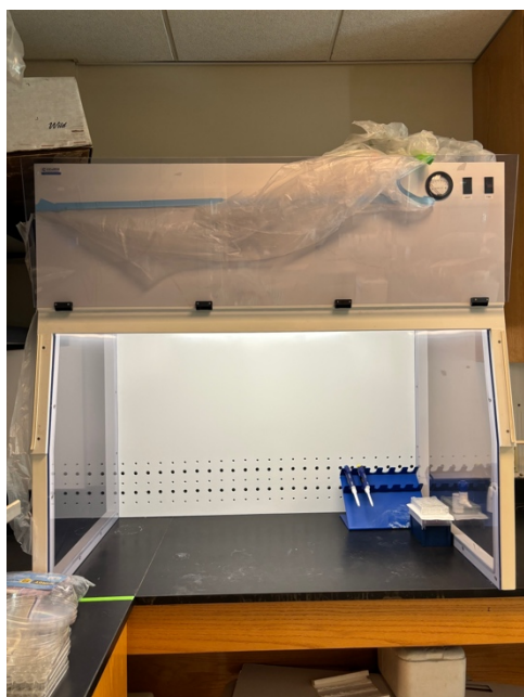
Figure S 5. Cleatech 24'' Portable Ductless Exhaust Fume Hood
