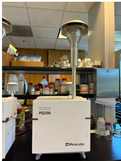
Figure S 4. MesaLabs PQ200 Ambient Air Particulate Sampler front exterior
