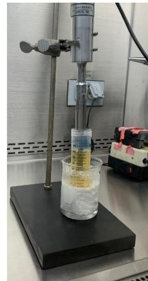
**Figure 6.** Sonication setup under tissue culture hood. The ultrasonic processor head is stabilized by ring stand. LCPAM solution is stabilized by a Styrofoam base and submerged in a beaker of ice.
