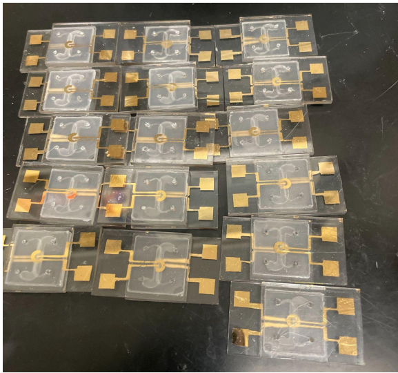
Figure 11. Completed \mu E-BBB devices without tubing and pogo pins
