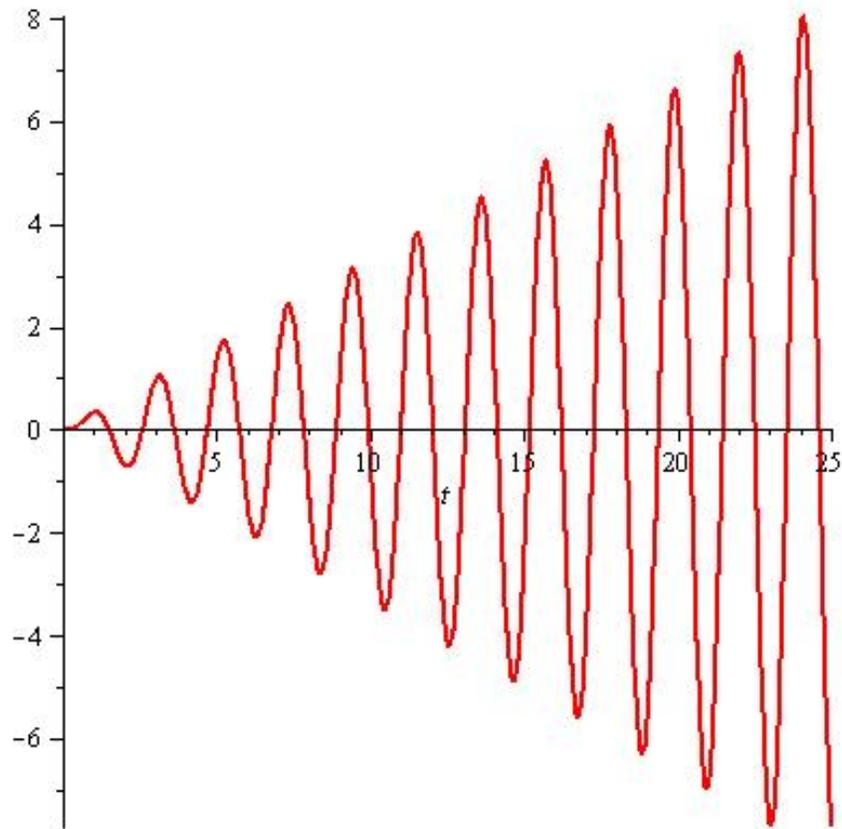
Figure 5: The aircraft wing's motion for  $0 \leq t \leq 25$  due to resonance and  $f_3(t)$
