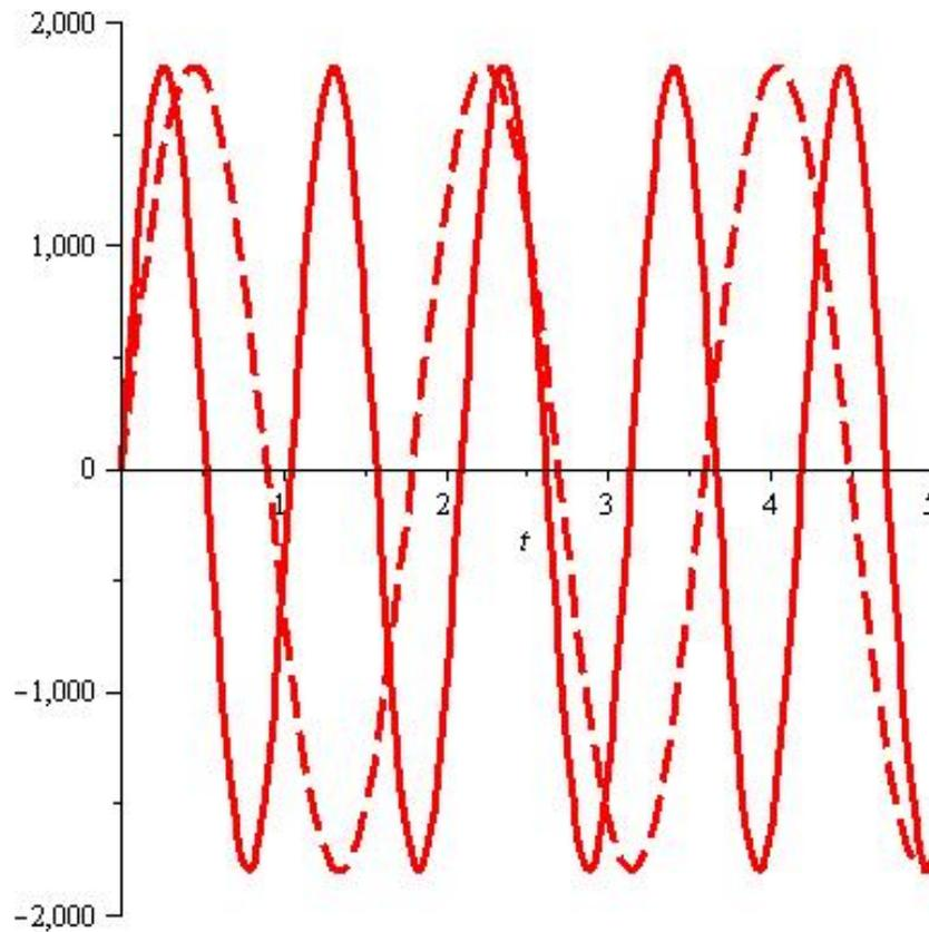
Figure 3: Two forcing functions (the dashed line is  $f_2(t) = 1800 \sin(3.5t)$ )
