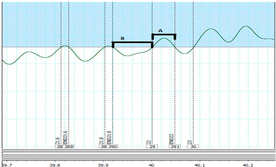
**Figure 2.** EMG time parameters measured for statistical analysis (horizontal line= threshold; y-axis= muscle electrical activity, measured in millivolts, x-axis= time measured in seconds; A= threshold period, B= length of time between each threshold period).
